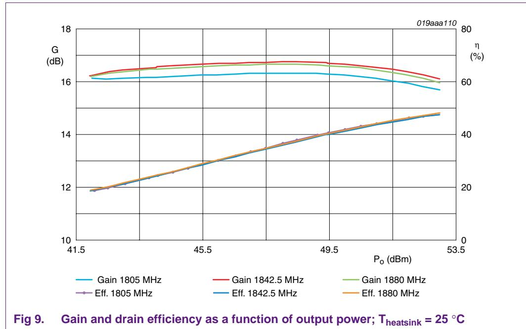
Fig 9. Gain and drain efficiency as a function of output power;  $T_{heatsink} = 25$  °C
