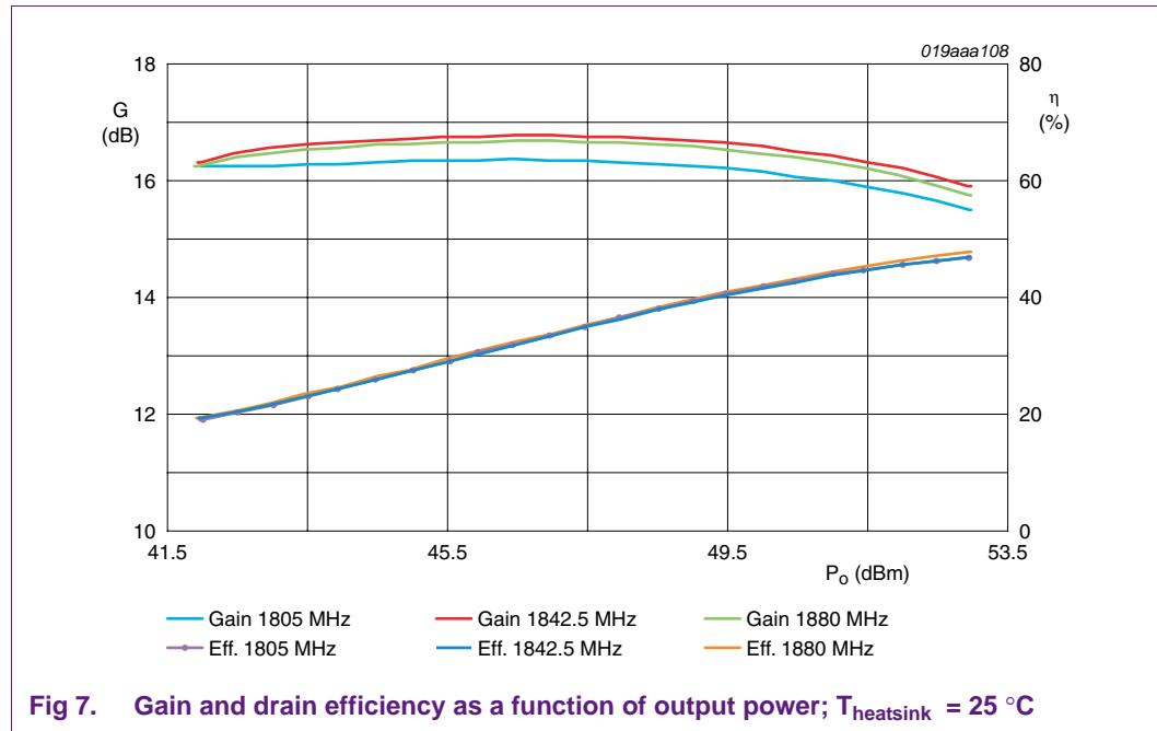
Fig 7. Gain and drain efficiency as a function of output power;  $T_{heatsink} = 25^\circ\text{C}$
