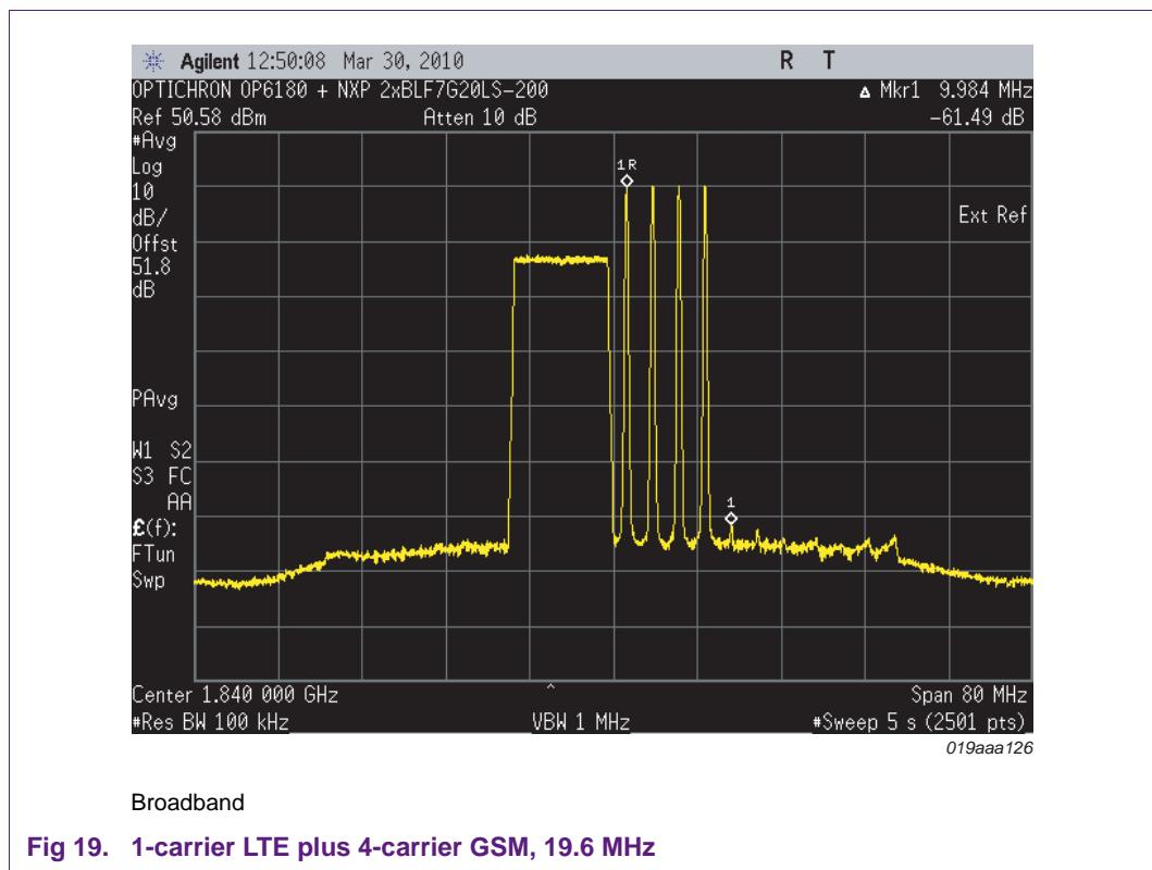
**Fig 19. 1-carrier LTE plus 4-carrier GSM, 19.6 MHz**
