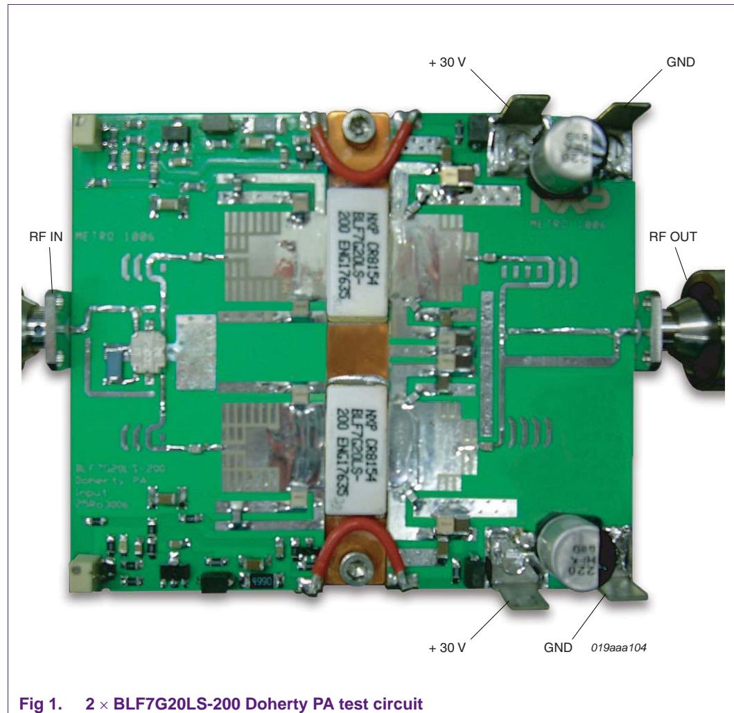
Fig 1. 2 × BLF7G20LS-200 Doherty PA test circuit
