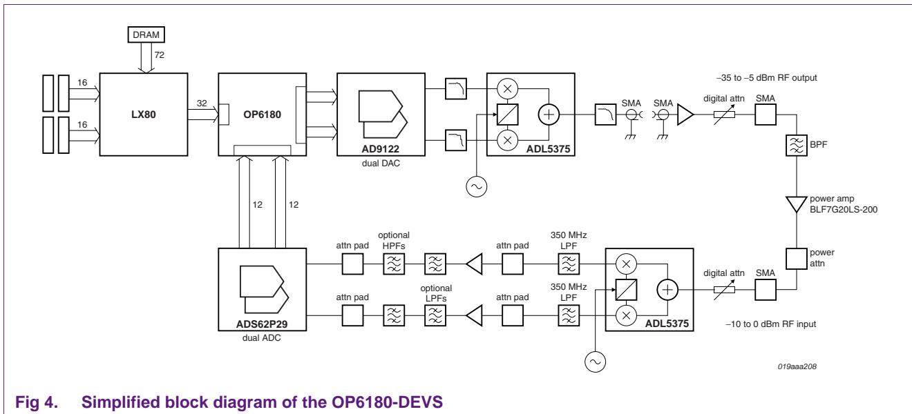
**Fig 4. Simplified block diagram of the OP6180-DEVS**
