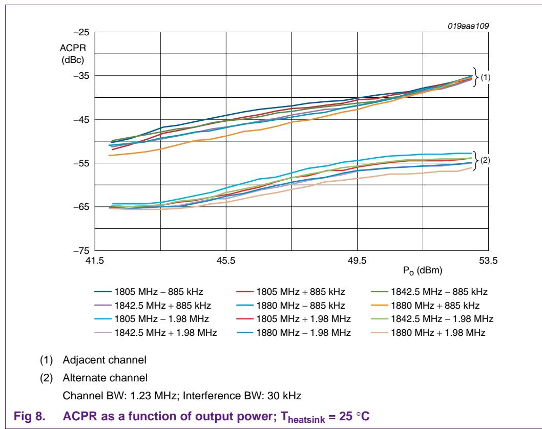
Fig 8. ACPR as a function of output power;  $T_{heatsink} = 25^\circ\text{C}$
